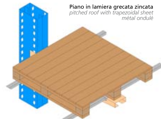
Rompitratta a filo zincata Load partitioning trusses Brise-trai
